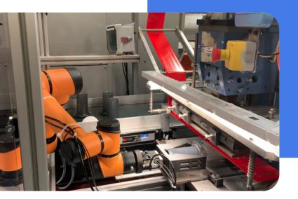
Westec assigned two RMOs, "Melvin" and "Nancy," to hot stamping and packaging Aeropress cylinders as they came out of the injection molds. That freed up six operators for other jobs, which gave Westec a crucial advantage when Aeropress approached it in 2021 with a \$600,000 job it had originally assigned to a facility in the Midwest.
